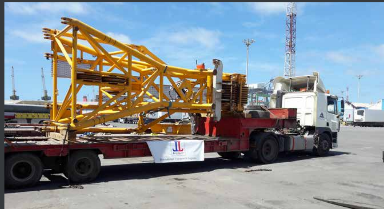
They loaded all the sections onto a MAFI Transport Systeme.
